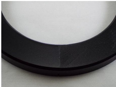
Figure 41 – Left side was sprayed with primer/filler, right side was not
