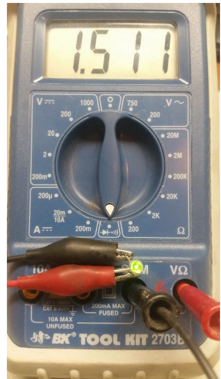
Figure 19 Using a meter to light an LED
