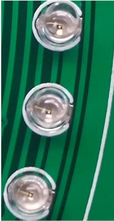
Figure 21 – Internal wires point the same way
