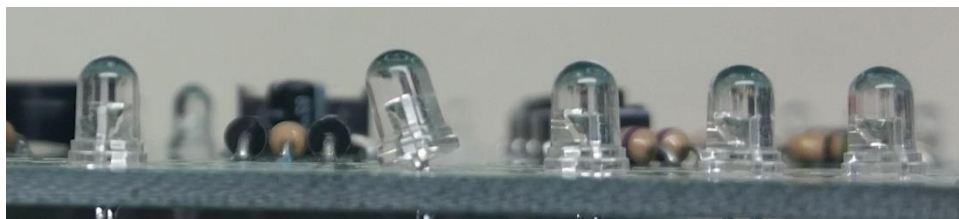
Figure 29 - LED not snug against board, needs rework
