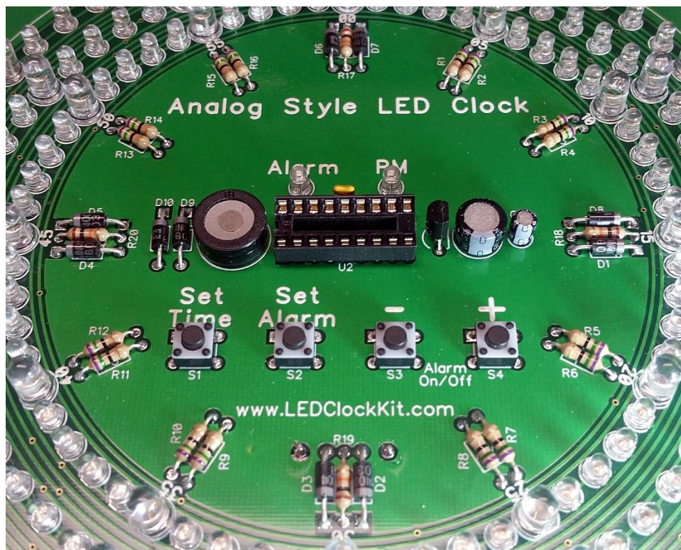
Figure 37 – Check the orientation of the parts
